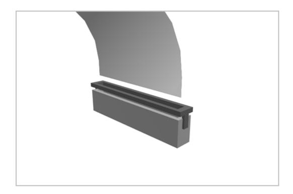
Figure 4-1. Removing a Cable from a ZIF Connector
